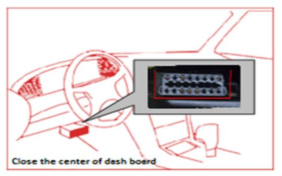
2. Plug the diagnostic connector into the vehicle' s DLC socket (It is suggested to use the OBD 2 extension cable to conn ect VCI connector and DLC socket.). For non-16PIN DLC socket, please select the corresponding non-16 pin connector a dapter, then plug the non-16pin end of the adapter into the DLC socket, and then connect the standard 16pinend VCI connector.
