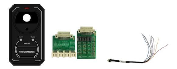
P001 Programmer is used for key transponder renewing and EEPROM reading and writing functions, the wiring of key r enewing (specific function operation is helpful in software) is as shown below.
