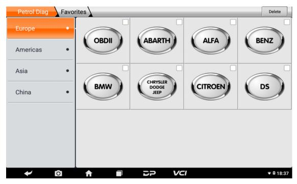
YSelect the corresponding menu to view the downloaded software of the machine configuration. OBDII software exists in e ach zone of diagnosis by default and lies in the first position. The following takes OBDII as an example to introduce how to start diagnosis. Click the "OBDII engine" icon under any regional menu, as shown in the figure:
