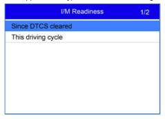
Depending on readiness test, one of these 2 screens will be present. Use the up and down arrow keys to scroll through data. Press the ESC key to exit.
