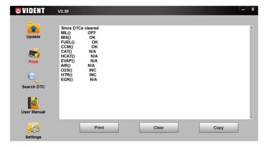
With the printer correctly connected, use the **Print** key to print the testing data. Press the **ESC** key to return to home screen.
