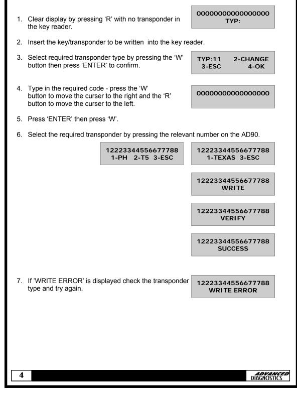
The Crypto Transponder Interface can be used in conjunction with the AD90 to copy first generation Philips crypto transponders (type 42) fitted to VAG group vehicles.
