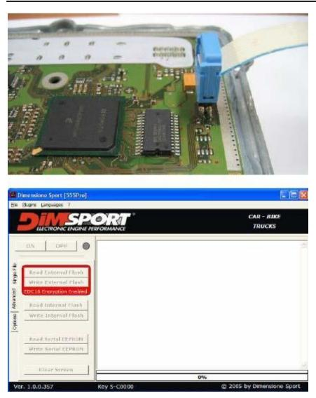
**BDM 100** allows also to create perfect copies of the whole software of an ECU (after having read the original ECU software).
